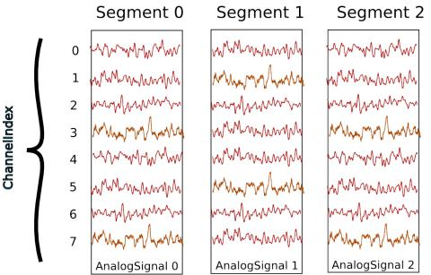
Segment and ChannelIndex objects provide two different ways to access the data, corresponding respectively, in this scenario, to access by **time** and by **space**.
